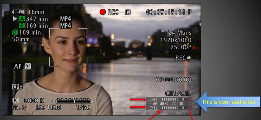
Often, you will use both of the two audio meters if you are recording stereo. Mono recording means only one channel.
