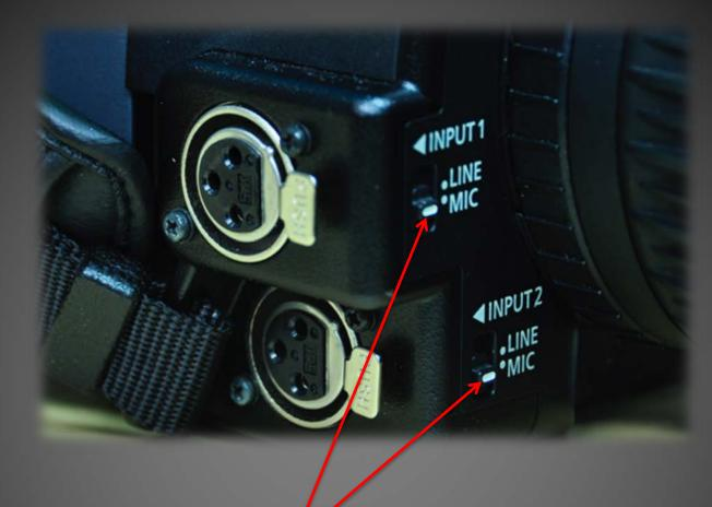
If the camera has a LINE/MIC switch, always set it to MIC if you are an external microphone. The LINE setting is for when you are connected to a mixing board, for example, and getting sound from a live event where the signal is stronger.\*
